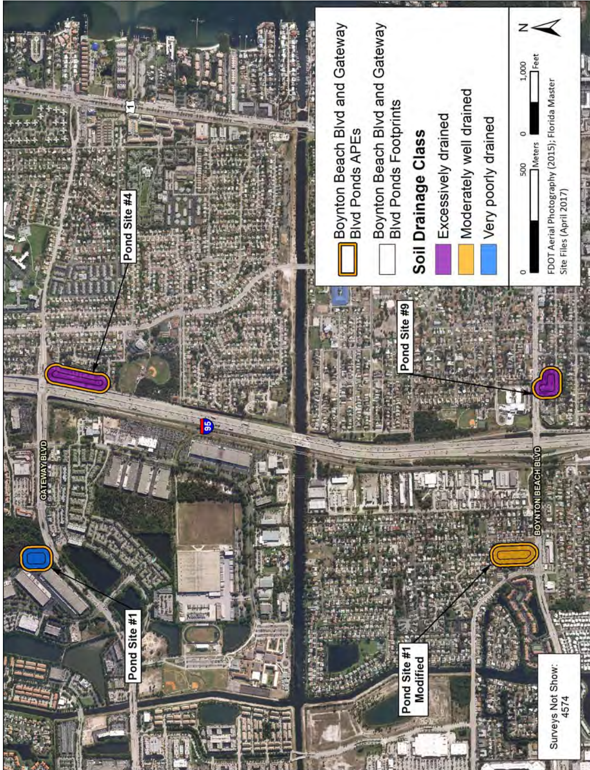
Figure 2. Soil drainage within the four proposed Boynton Beach Boulevard and Gateway Boulevard Ponds.
